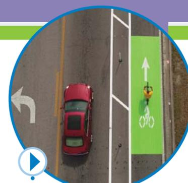
The demonstration project reduced the number of travel lanes and added separated bike lanes along both sides of the street and contributed to a **50%** increase in bicycle usage.
